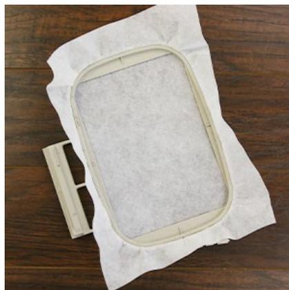
Hoop a piece of tearaway stabilizer, and load the embroidery file (not a dieline file) onto the machine.
