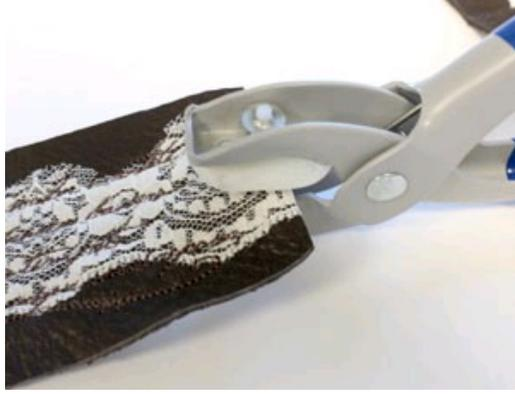
Before you add your first piece, wrap the edge of your lace (if you added it) around the end of the leather, so the end can be secured by the clasp. Place the tool over your desired spot and clamp down hard. You should be applying this so the shiny button piece will end up on the same side as your embroidery.
